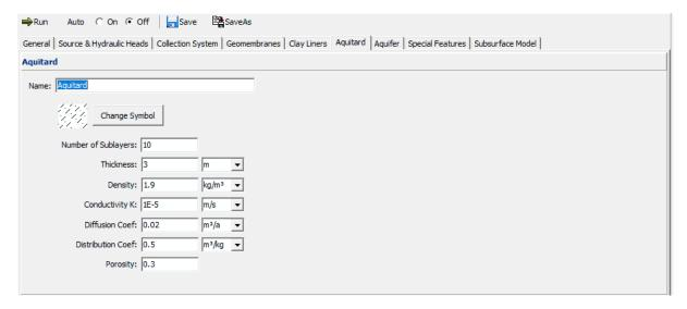
The parameters for the aquitard are specified on the Aquitard tab.
