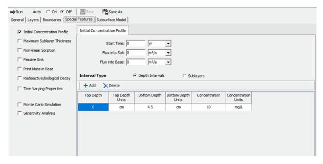
To specify the initial concentration profile, check the Initial Concentration Profile box on the Special Features tab.
