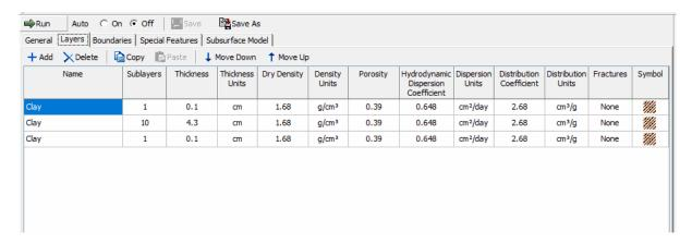
There are no fractures in these layers. For pure diffusion even if there were fractures it should be modelled as if the soil was unfractured, since there would be no flow in the fractures for pure diffusion.
