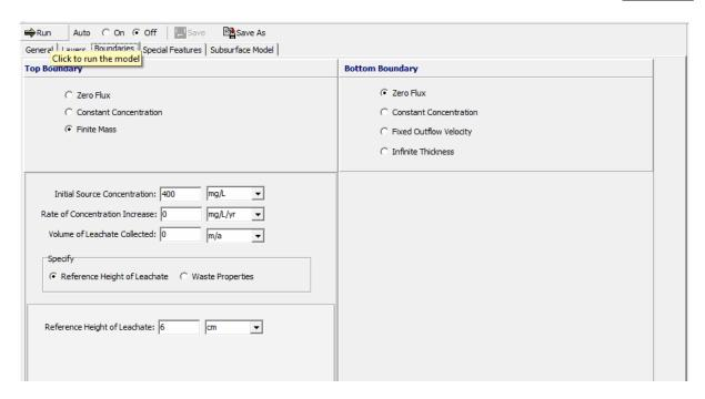
In this example, the top boundary has a finite mass and the bottom boundary is represented as a zero flux layer.
