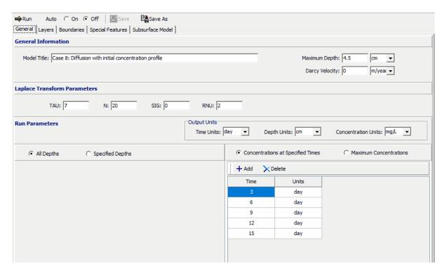
On the General tab the Darcy velocity is set to zero for pure diffusion. The concentrations can either be calculated at specified times or the time of the maximum concentration can be found. In this example the concentrations will be calculated at 5 times: 3, 6, 9, 12, and 15 years.
