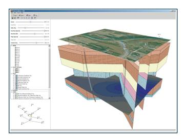
StrataExplorer is an application suite for subsurface mapping, data management, and resource evaluation. The program can be used to evaluate contaminants, soil and rock properties, minerals, oil and gas deposits, and oil sands. It is ideal for the environmental, geotechnical, mining, oil sands, and petroleum industries.
